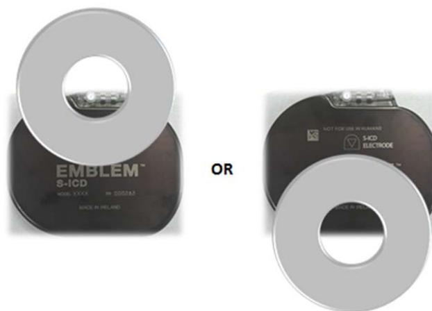
Figure 2. Magnet placement for EMBLEM
