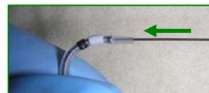
Figure 2. Guide wire insertion into electrode end of lead.
